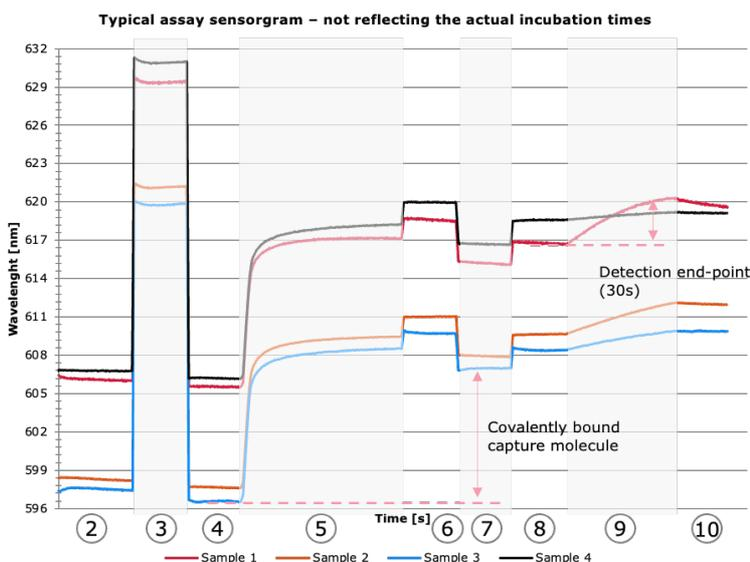
Figure 2: A typical FO-SPR sensorgram showing all steps of covalent immobilization of antibodies (5-7) and subsequent TRA detection (9) using the label-free bioassay approach as described in the run sequence of Table 2. Recordings shown represent 4 different concentrations of Trastuzumab applied in step (9).
