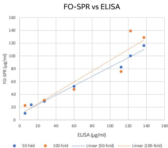
Figure 4: Evaluation of the FO-SPR assay with crude bioreactor samples compared to the results from the anti-IgG ELISA test. Data plotted as undiluted initial sample concentrations. Pearson correlation coefficient: 0.992 at 50-fold dilution and 0.928 at 100-fold dilution.
