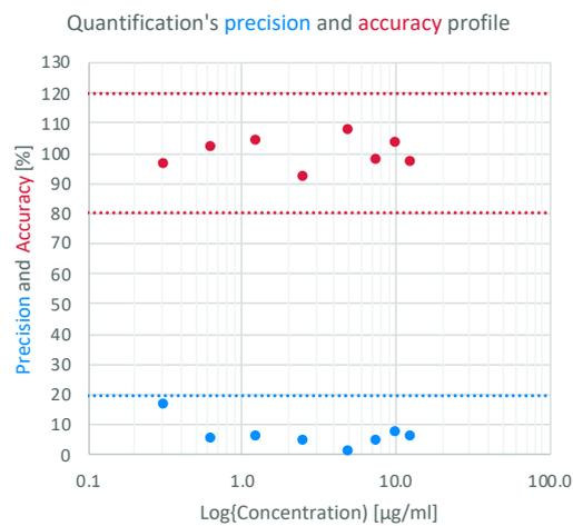
Figure 3: Top: Calibration curve for spiked TRA in buffer-lysate. Error bars represent standard deviation. Bottom: precision and accuracy profile plot for the calibrator samples.
